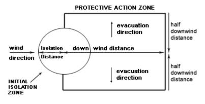
From IERG (Canada/Australia) Isolation Distance **Downwind Protection Distance 10 meters**
