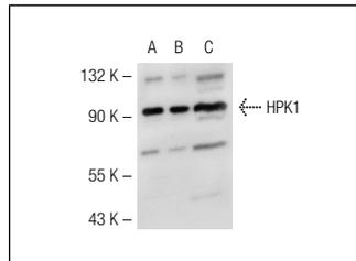
HPK1 (H-200): sc-25414. Western blot analysis of HPK1 expression in non-transfected 293T: sc-117752 (A), mouse HPK1 transfected 293T: sc-126974 (B) and BJAB (C) whole cell lysates.
